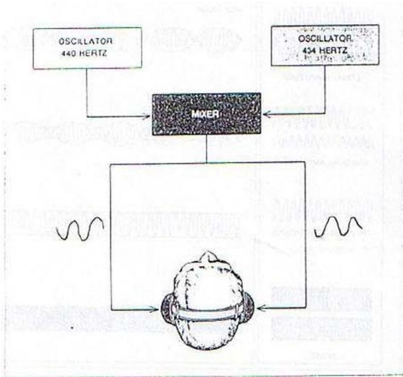
**EXPERIMENTAL METHOD** for generating monaural beats uses two electronic oscillators and a network, here called a mixer, to combine their outputs. Each ear hears a composite signal; the beats can be heard with one ear or both. With the oscillators tuned to the frequencies shown, six beats per second (440 hertz minus 434 hertz) would be perceived.
