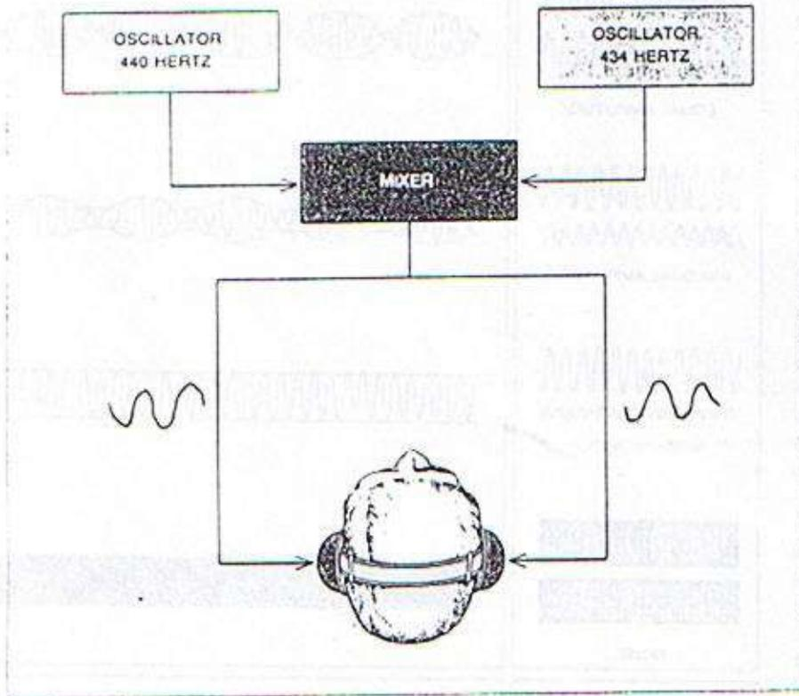
EXPERIMENTAL METHOD for generating monaural beats uses two electronic oscillators and a network, here called a mixer, to combine their outputs. Each ear hears a composite signal; the beats can be heard with one ear or both. With the oscillators tuned to the frequencies shown, six beats per second (440 hertz minus 434 hertz) would be perceived.
